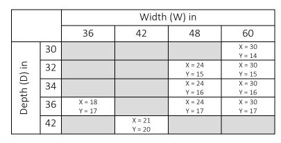
Tolerances: W = +/-1/8"; D = + curb tile thickness; X = +/-1/8"; Y = +/-1/8"
